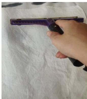
Figure 2. Coating with neat PLA Solution
